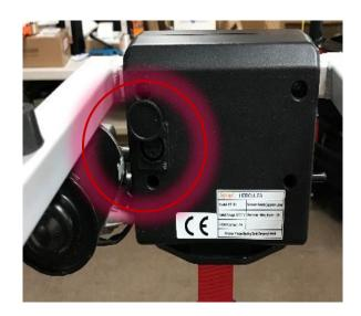
7) Attach the other end of the power cord to the port on the Hercules Lift Motor (as shown in the red circle in the photo to the left).
