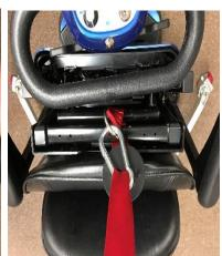
10) To raise the scooter off the ground, make sure the brake is engaged and push up on the dual switch located on the motor of the scooter lift. See Photo below
